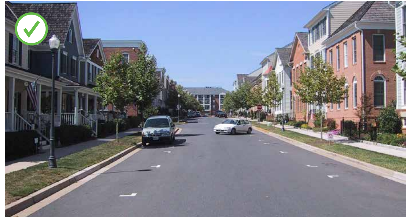
A good example of a streetscape with on-street parking and a landscape strip separating the sidewalk from the curb.
