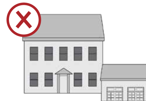
Garage in extended side wing, front-facing
