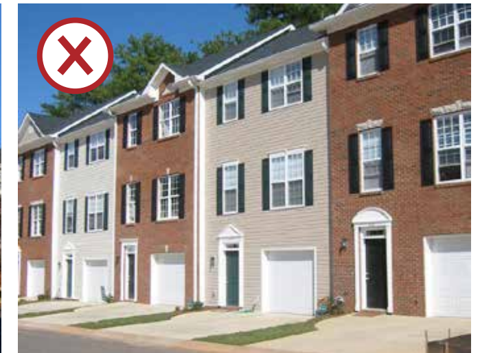
Using the same materials and window and door placements on more than a few facades at a time can contribute to a "flat" appearance.
