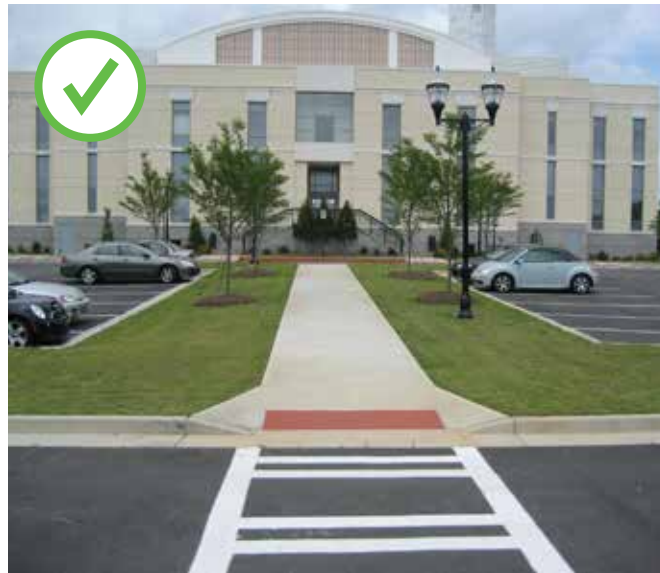
A walkway connects from the public sidewalk to the primary building entrance.
