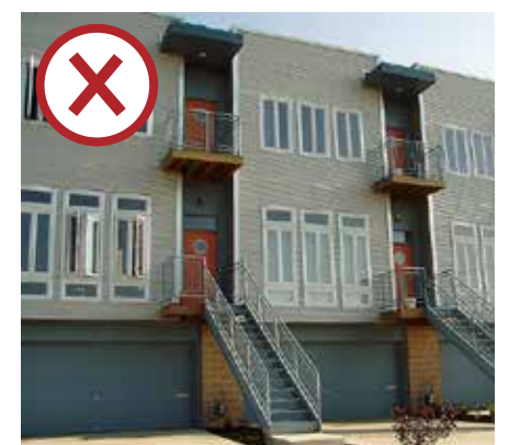
Doors wider than 10 feet can make a front facade look "flat" and uninteresting.
