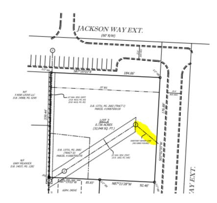
Show the sewer line located in the area highlighted below. This sewer line must be located in an
